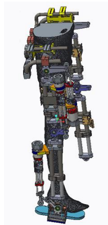
Fig. 1 Illustration of the developed scalable lower extremity exoskeleton model
